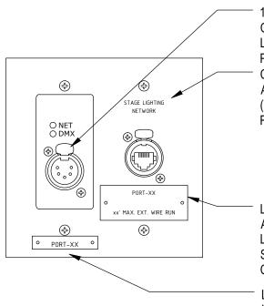
1-PORT ETHERNET-TO-DMX512 OUTPUT NODE WITH INDICATOR LEDS. NODE TO BE POWERED VIA PoE
